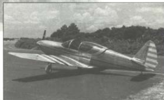
With 420 shp, Lopresti Piper's prototype Allison turboprop Swift has power to burn. Note the absence of draggy exhaust pipes.
